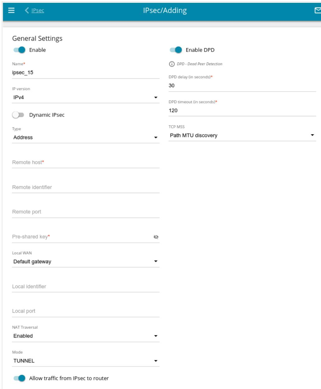
Figure 133. The page for adding an IPsec tunnel. The **General Settings** section.
