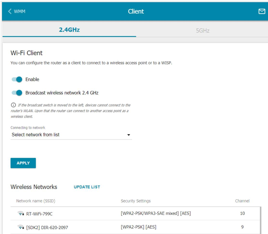
Figure 108. The page for configuring the client mode.
