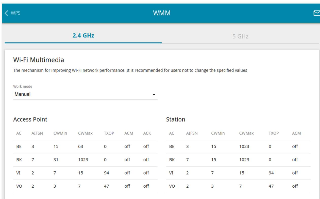
Figure 106. The page for configuring the WMM function.
