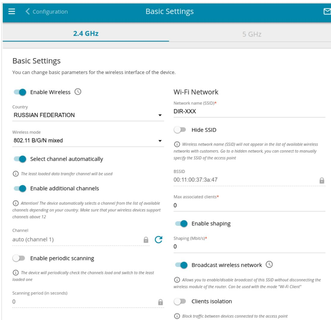
Figure 98. Basic settings of the wireless LAN in the 2.4GHz band.
