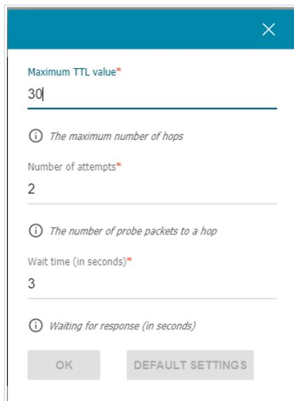
Figure 157. The **System / Traceroute** page. The additional settings window.
