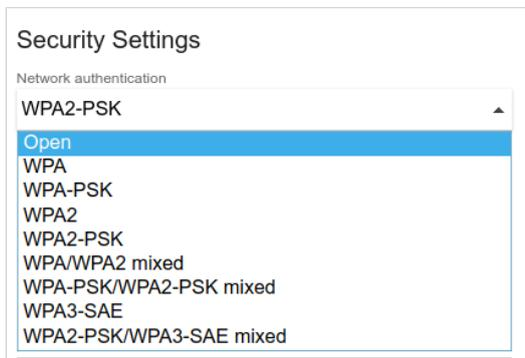
Figure 100. Network authentication types supported by the router.
