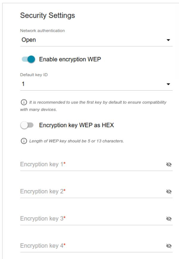
Figure 101. The **Open** value is selected from the **Network authentication** drop-down list.
