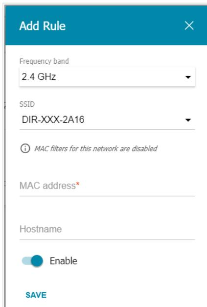
Figure 113. The window for adding a rule for the MAC filter.
