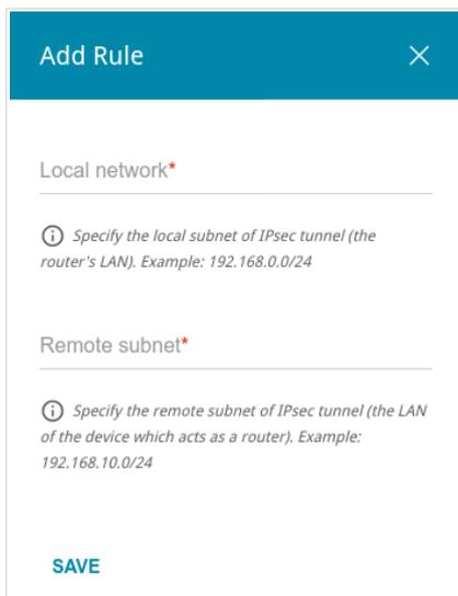
Figure 135. The page for adding an IPsec tunnel. The window for adding a tunneled network.
