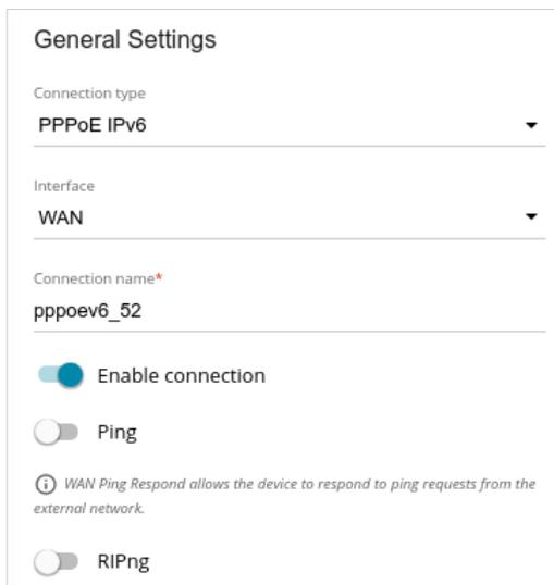
Figure 82. The page for creating a new **PPPoE IPv6** connection. The **General Settings** section.
