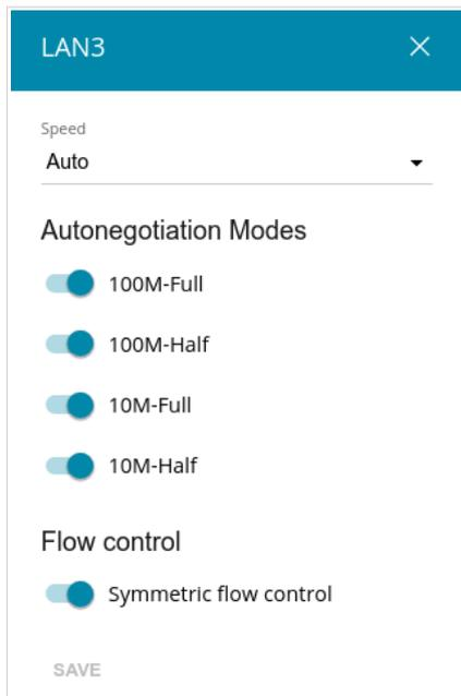
Figure 122. The window for changing the settings of the router's port.
