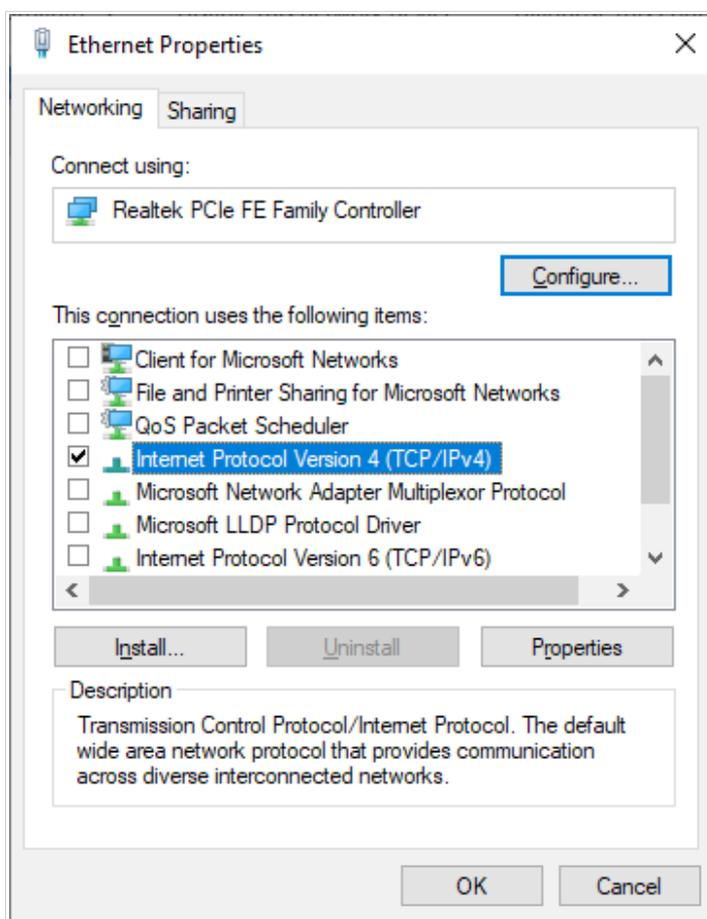
Figure 11. The local area connection properties window.
