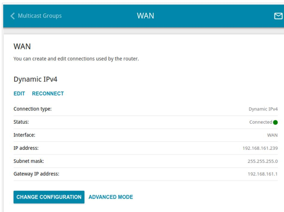
Figure 66. The **Connections Setup / WAN** page. The simplified mode.
