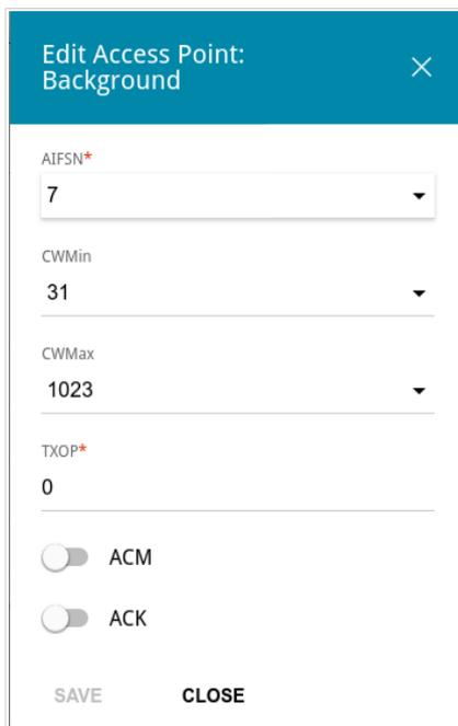
Figure 107. The window for changing parameters of the WMM function.
