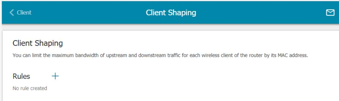
Figure 109. The **Wi-Fi / Client Shaping** page.
