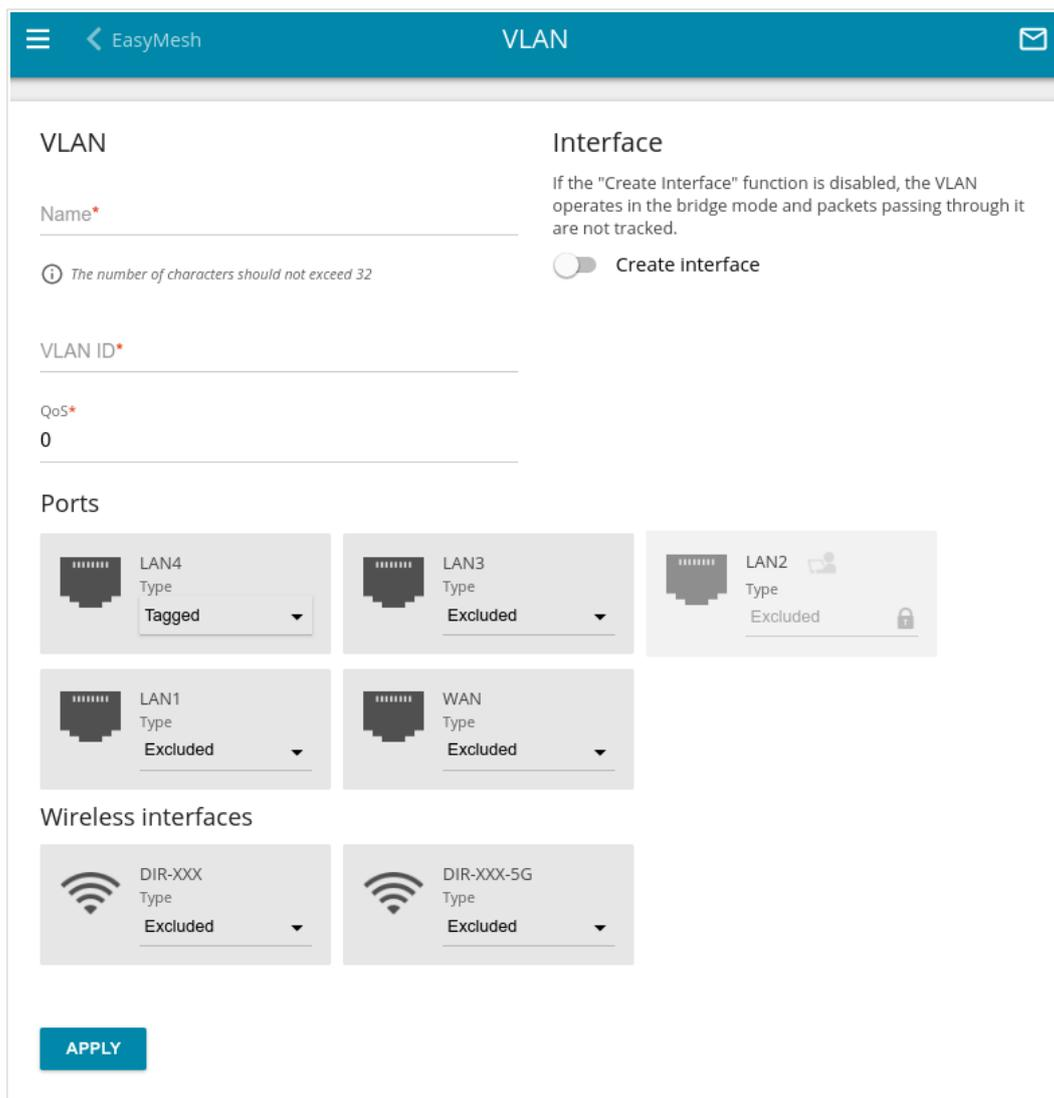
Figure 117. The page for adding a VLAN.
