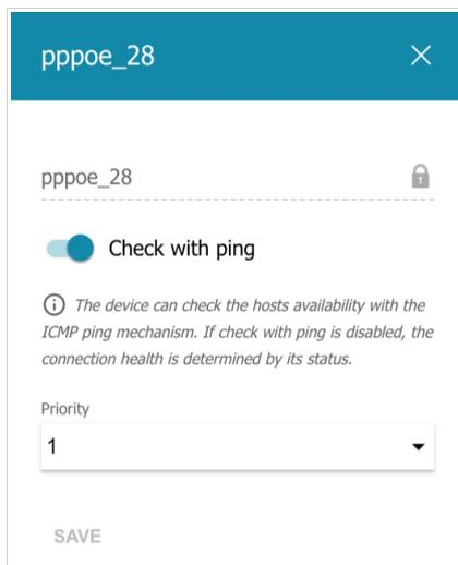
Figure 97. The window for changing the priority of a connection.
