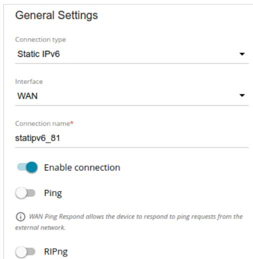
Figure 71. The page for creating a new **Static IPv6** connection. The **General Settings** section.
